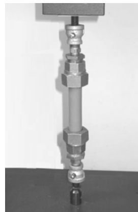
MUNICIPEX at start of test; no load
